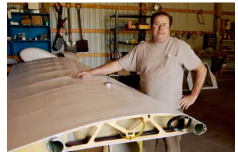
The wings contain the 26-gallon fuel tank. Fuel is consumed at a rate up to 5 gal/hr.
