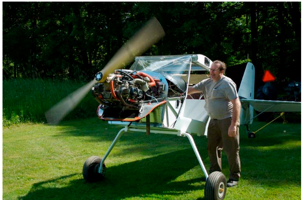
Gerry Jantzi runs his newly acquired Rotax engine for a demonstration. The aircraft is shown here without the wings or cowling or wheel fairings. This twin seater lifts off, at speeds as low as 72 kph (45 mph). The 'tail-dragger' wheel configuration is trickier on the ground.
