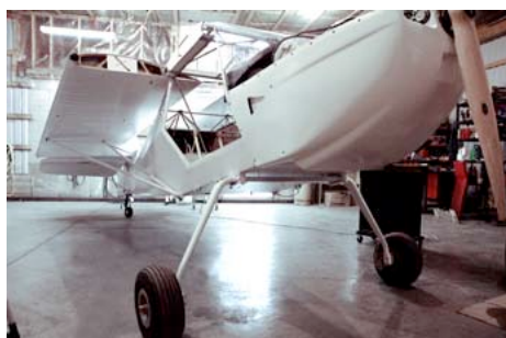
Here the wings are mounted to the aircraft. They are pivoted back to store or transport.
