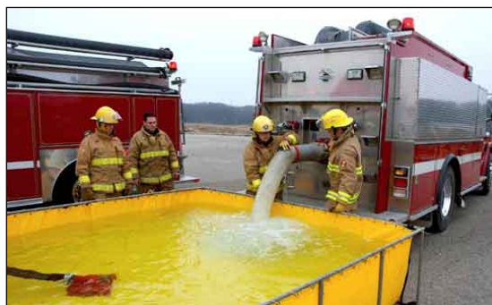
Pumpers fill up this porta-tank, a swimming pool-like reservoir. They can be cascaded for more capacity. Each holds 1500 gallons.
